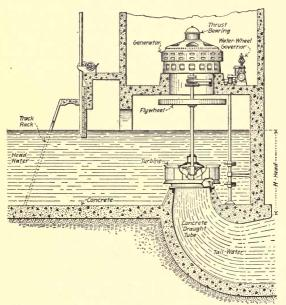
Fig. 293.—Low-head, vertical water wheel generator station. (Electrical Machinery Company.)
